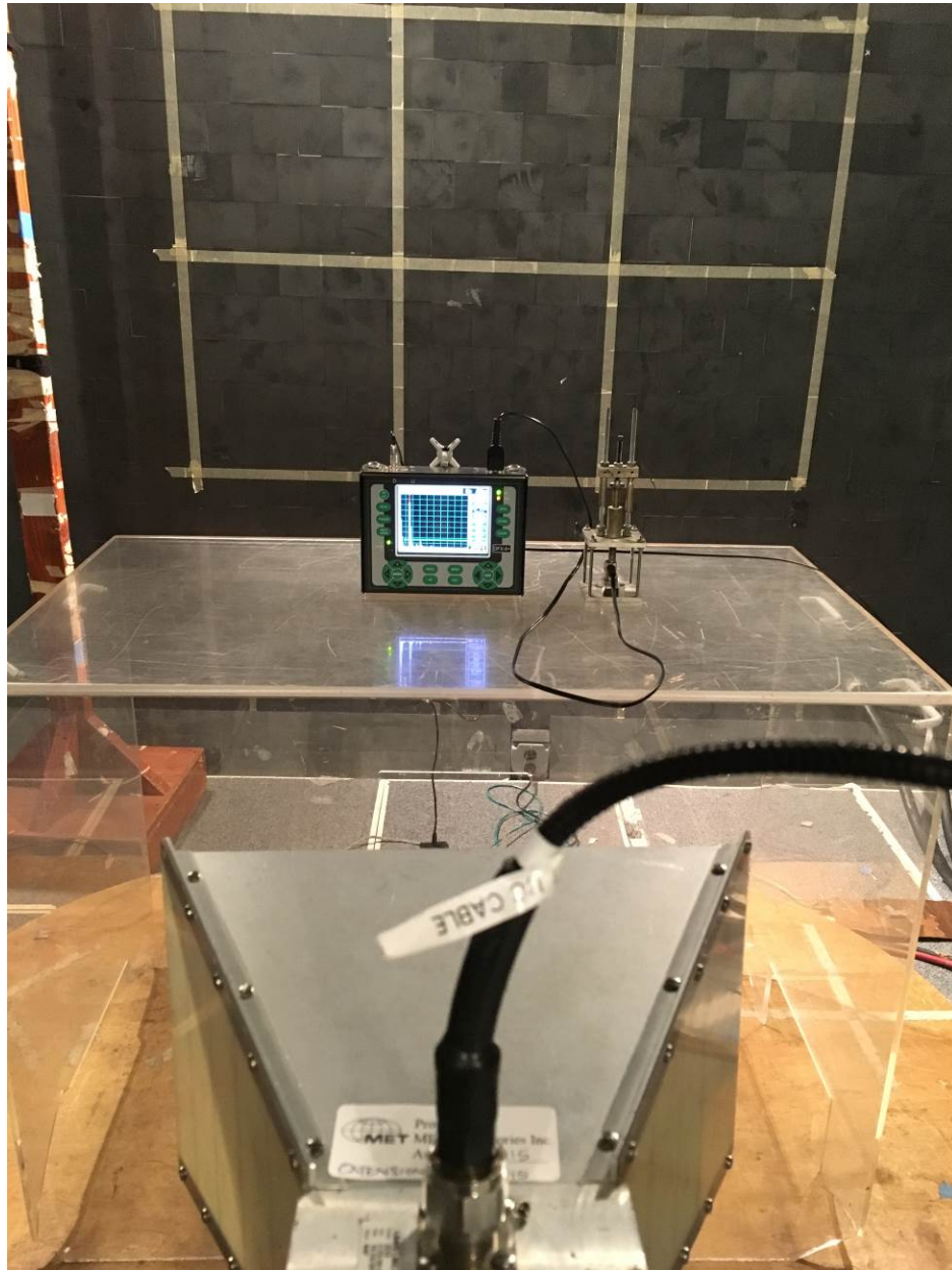
Photograph 30. RI (1 – 2.7 GHz) Test Setup (DFX-8)
