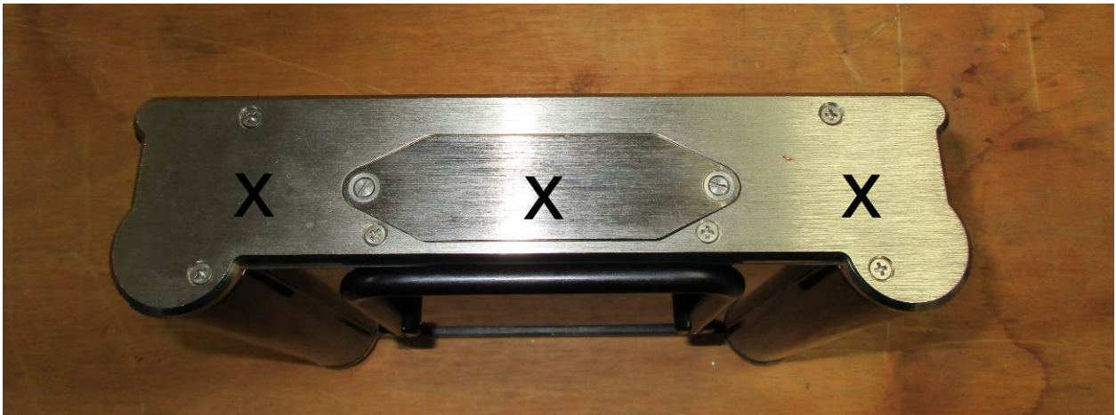
Photograph 21. ESD Test Points – Bottom of EUT (DFX-8)
