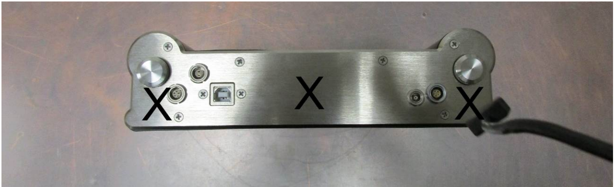
Photograph 25. ESD Test Points – Top of EUT (Max II)
