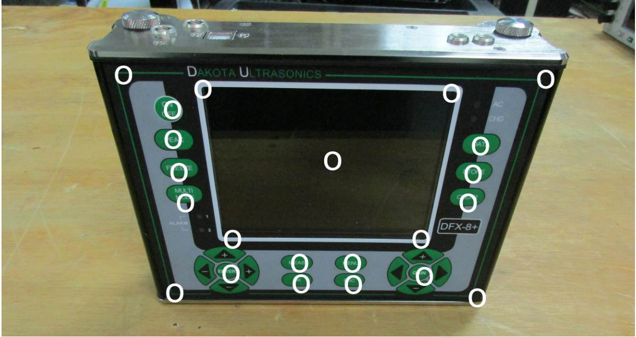
Photograph 17. ESD Test Points – Front of EUT (DFX-8)
