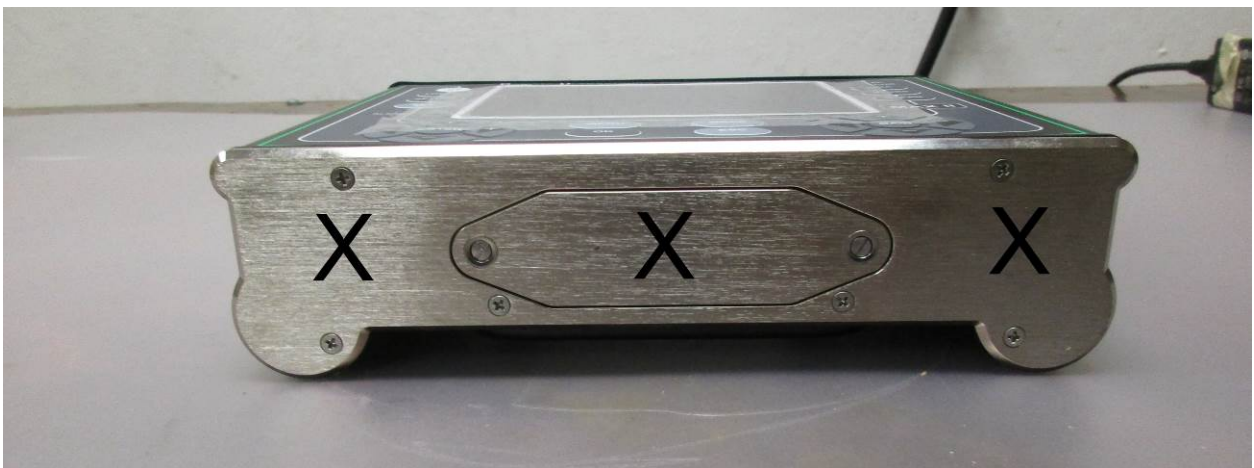
Photograph 26. ESD Test Points – Bottom of EUT (Max II)
