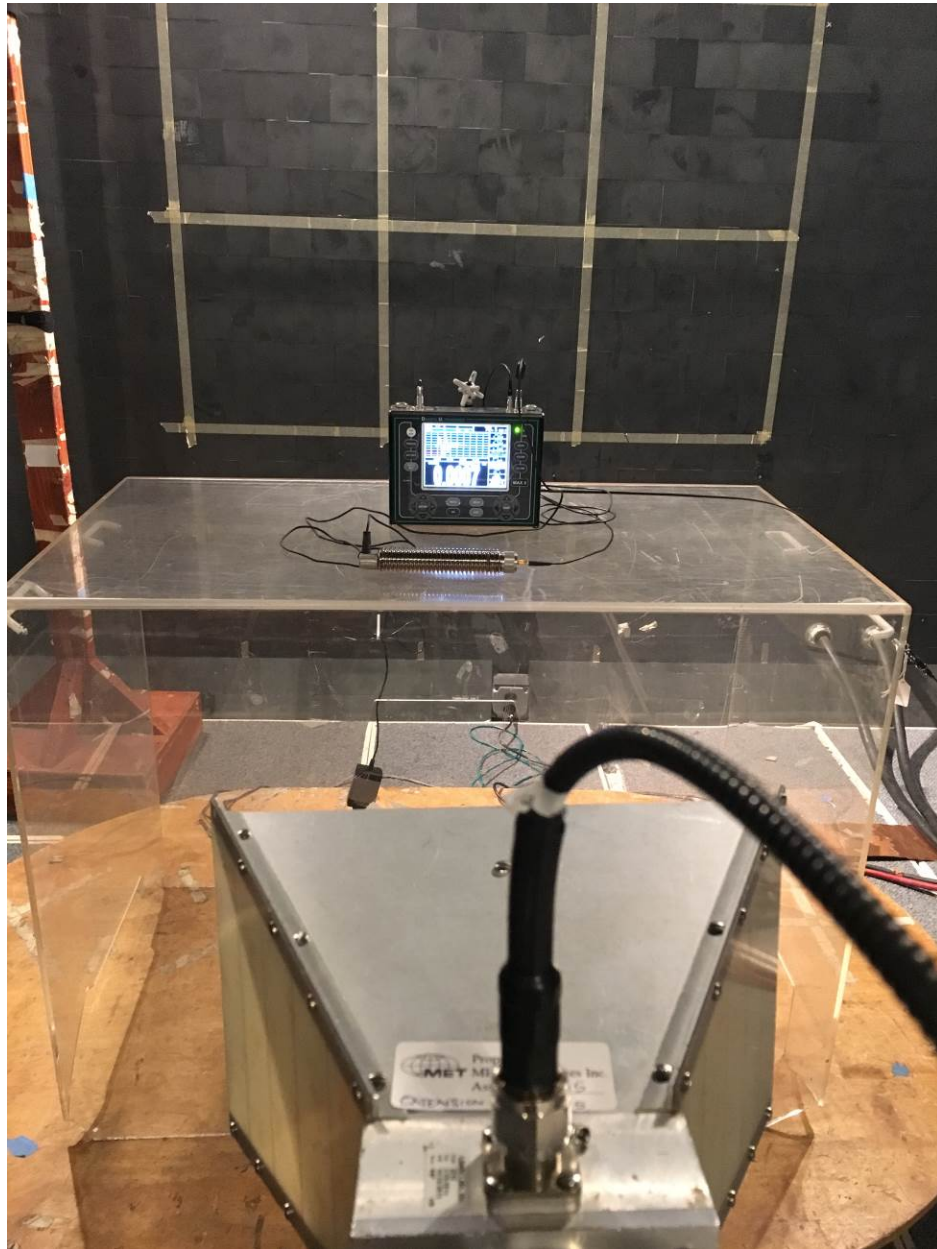
Photograph 32. RI (1 – 2.7 GHz) Test Setup (Max II)
