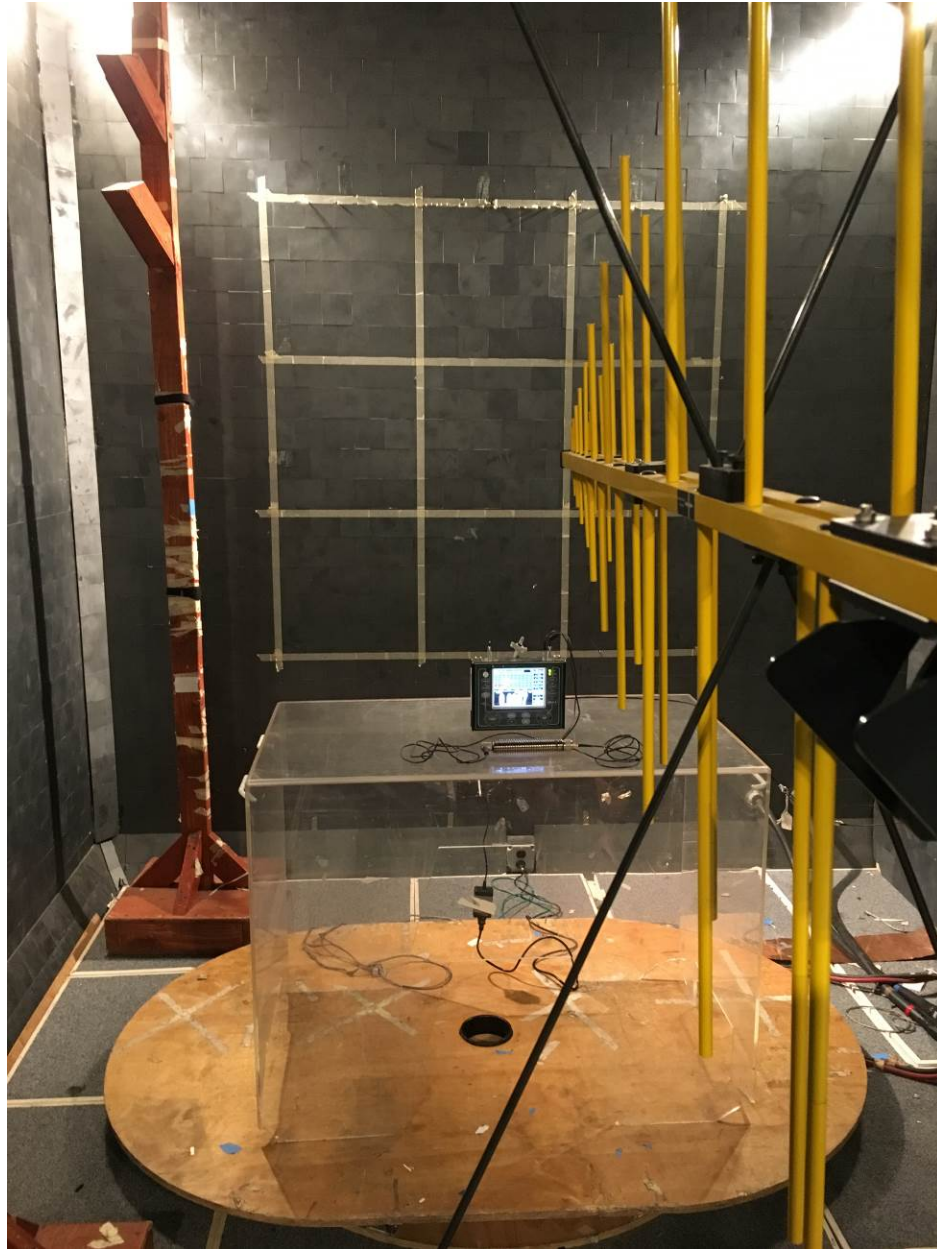
Photograph 31. RI (80 MHz – 1 GHz) Test Setup (Max II)
