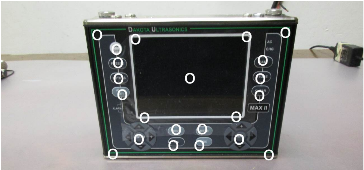
Photograph 22. ESD Test Points – Front of EUT (Max II)
