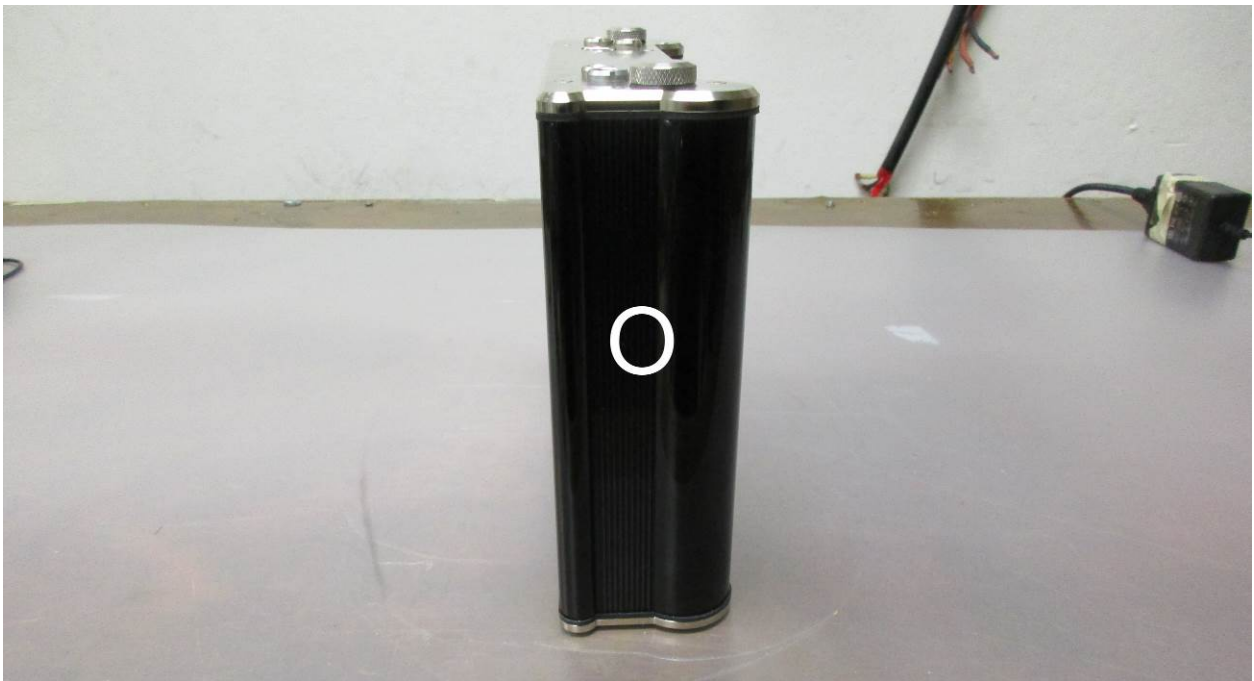
Photograph 23. ESD Test Points – Right of EUT (Max II)
