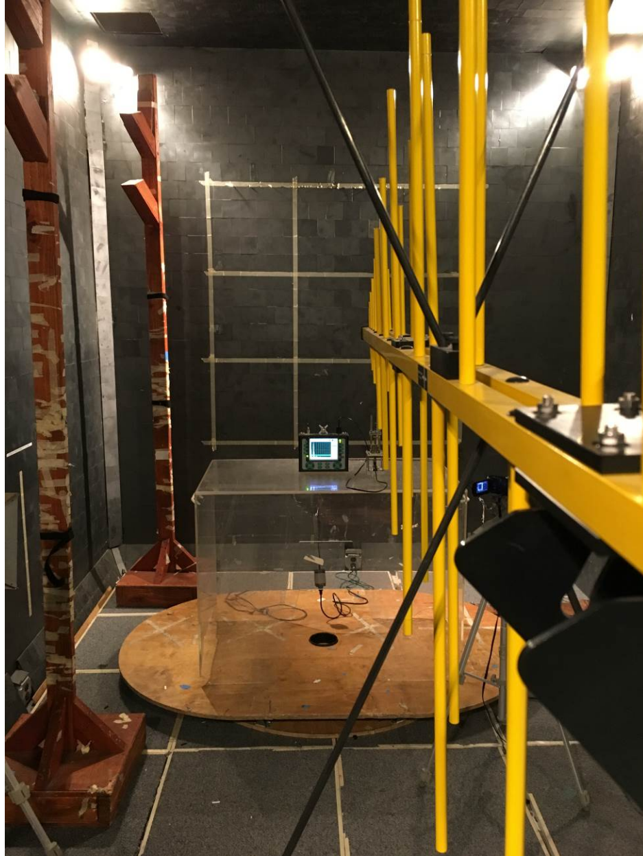
Photograph 29. RI (80 MHz – 1 GHz) Test Setup (DFX-8)
