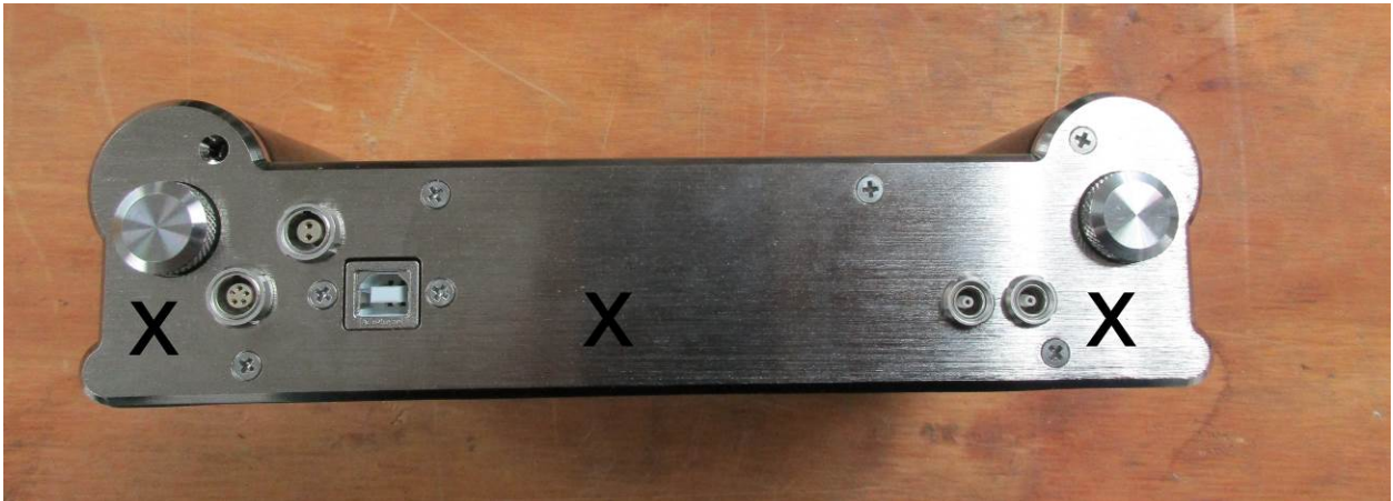
Photograph 20. ESD Test Points – Top of EUT (DFX-8)
